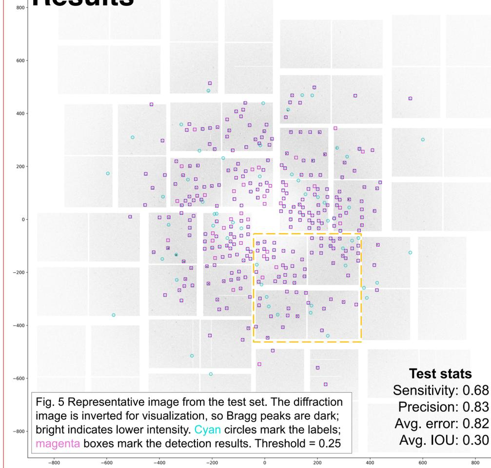
Fig. 5 Representative image from the test set. The diffraction image is inverted for visualization, so Bragg peaks are dark; bright indicates lower intensity. Cyan circles mark the labels; magenta boxes mark the detection results. Threshold = 0.25
