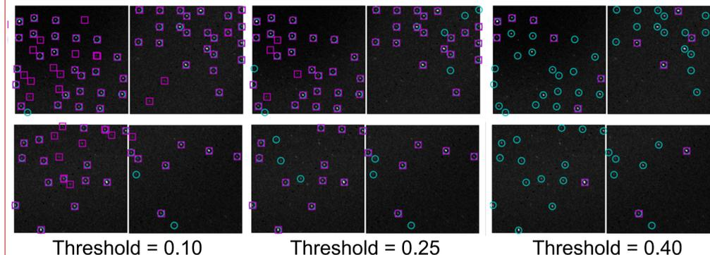
Fig. 6 Zoom-in of the yellow box in Fig. 5. Higher detection threshold gives better precision but lower sensitivity. Note that many "false positives" are actually Bragg peaks that weren't labelled.
