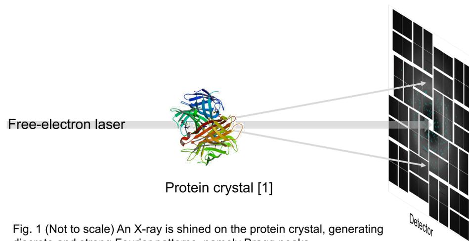
Fig. 1 (Not to scale) An X-ray is shined on the protein crystal, generating discrete and strong Fourier patterns, namely Bragg peaks
